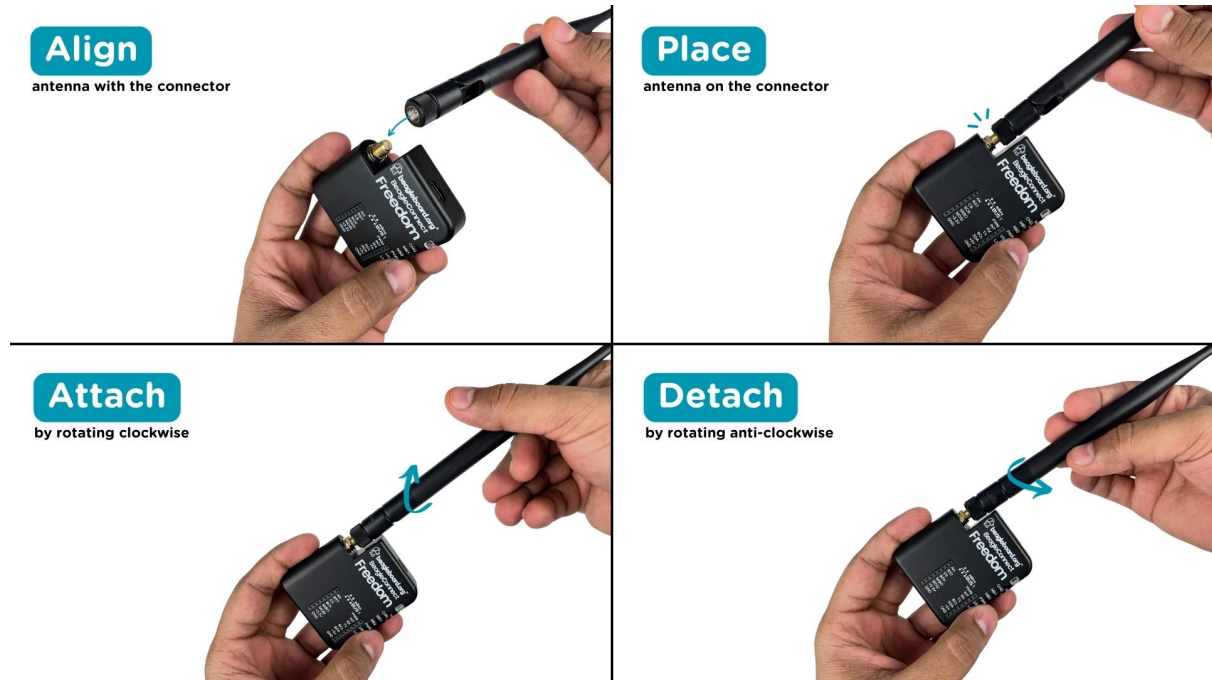
Fig. 10.1: Attaching antenna to BeagleConnect Freedom
